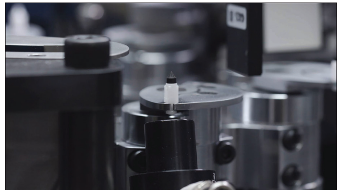
Embedded Teledyne DALSA iInspect Express software assesses each image to ensure that all measurements meet critical dimension standards and are within a tolerance of .08 mm. Any valve assemblies that don't meet customer standards are ejected through a vacuum and discarded.
