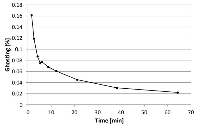
Figure 9 Ghosting after covering half of the detector with lead and irradiating with 15 mGy X-ray exposure.
