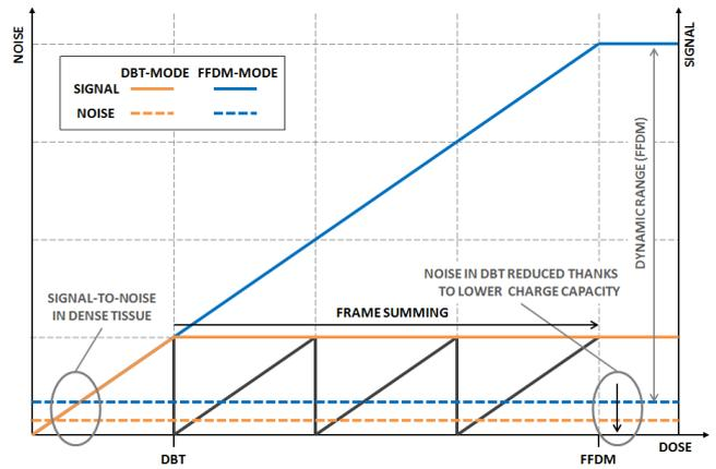
Figure 2 FFDM & DBT modes using frame summing
