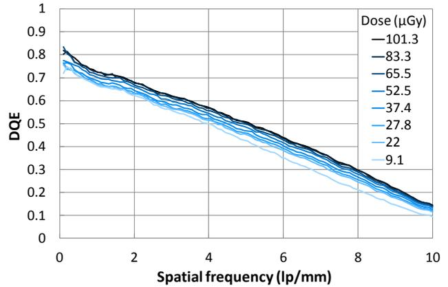
Figure 7 The measured DQE performance as function of dose in DBT mode at 28 kV, W/Rh.
