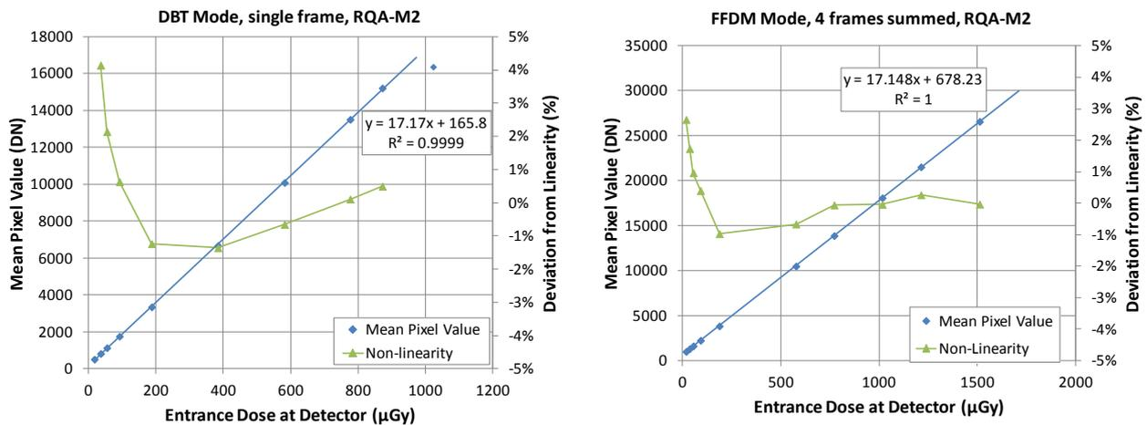
Figure 3 Blue curve shows the sensitivity in DBT (left) and FFDM (right) mode measured at RQA-M2. Green curve shows the deviation from a linear fit through the measurement points.
