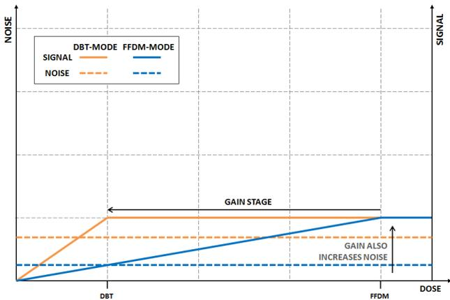
Figure 1 FFDM & DBT modes using gain switch
