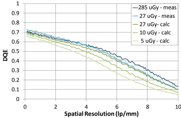
Figure 6 The measured (blue) and modeled (green) DQE performance in DBT mode at RQA-M2.
