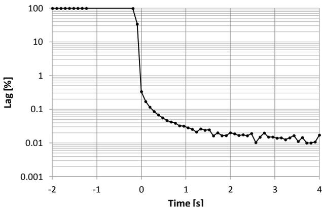
Figure 8 Lag after 3 mGy X-ray exposure during 2s.
