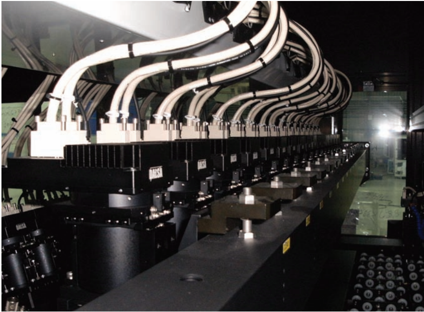
Figure 4. This automatic optical inspection system for color filters uses Teledyne Dalsa's ES-8k/7- \mu\text{m} 32-stage TDI cameras. The single-pass system uses 34 cameras. Courtesy of Utechzone Co. Ltd.
