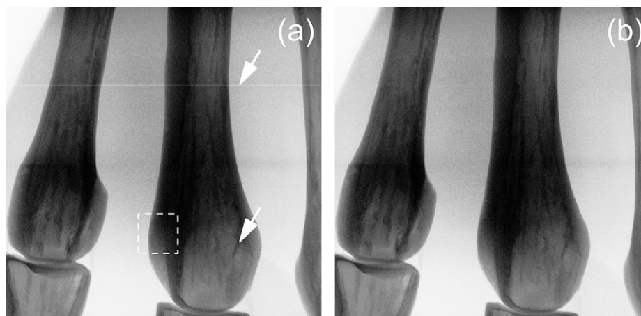
Fig. 6. Example of defective-pixel correction in digital radiography with the defective pixel map. (a) An image of hand phantom obtained from the CMOS detector. (b) Defect-corrected image by adaptive median filtering operation based on the defective pixel map.
