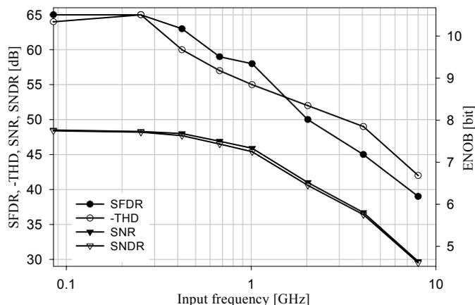
Fig. 11: Measurement result of the time-interleaved ADC at 1.35 GS/s
