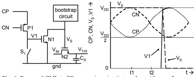
Fig. 6: Proposed CML to SE conversion circuit, together with waveforms
