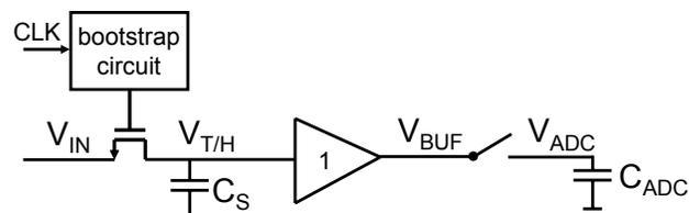
Fig. 2: Overview of 1 of the 16 T/H channels
