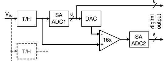
Fig. 8: Overview of the sub-ADC architecture (1/16 of total ADC)
