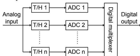
Fig. 1: time-interleaved ADC architecture
