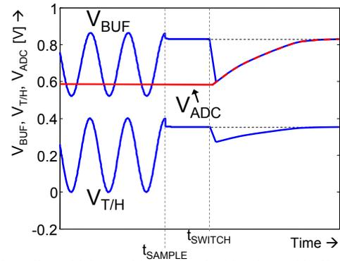
Fig. 5: Sampling a high speed input signal with enhanced buffer bandwidth
