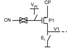
Fig. 7: Circuit enabling the use on a multi-phase clock
