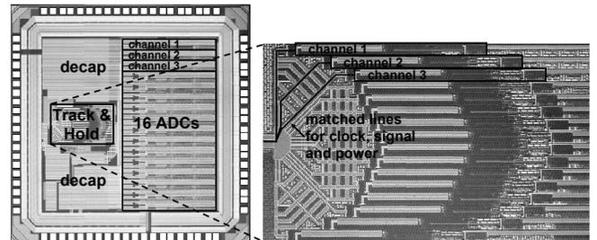
Fig. 9: Photograph of the time-interleaved ADC and zoom-in on T/H
