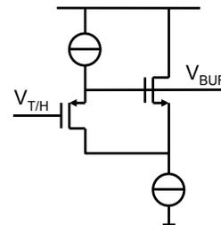
Fig. 3: High-linearity input buffer
