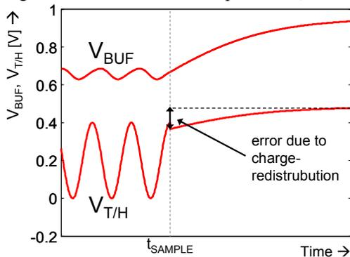
Fig. 4: Sampling a high speed input signal with limited buffer bandwidth
