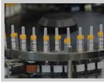
Fill level on disposable vaccine injection syringes
