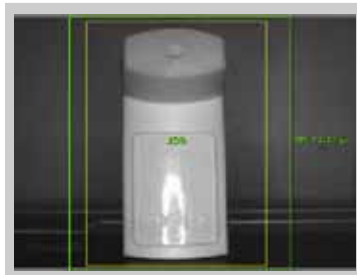
Surface quality and cap presence on canister
