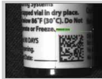
Product traceability using 2D code reader
