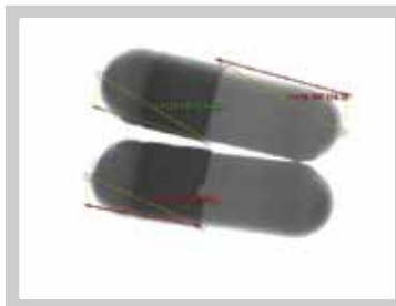
Capsule size checking using measurement tools
