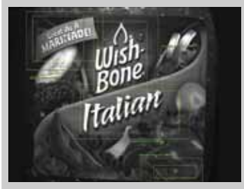
Label presence, placement and integrity
