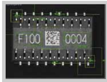
Verify the number of pins and identification markings on an IC
